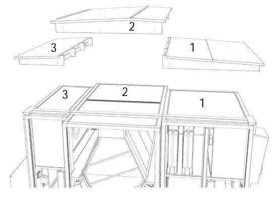
Roof blocks on the units 9000 MultiEco-N and 11000 Multi-N
