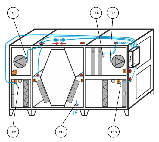
Connection of temperature sensors and condensate drain heating
