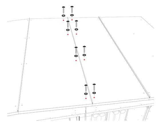
5. Attach side plates of roof blocks to the side of unit casing. Use holes that are drilled in the side plates. Use tek screws star 4x16mm (part of delivery). Attach the tek screws directly into the casing all around the unit.
