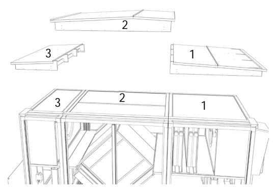
Roof blocks on the units 12100 Basic-N and 15100 Basic-N, 7500 MultiEco-N and 10000 Multi-N
