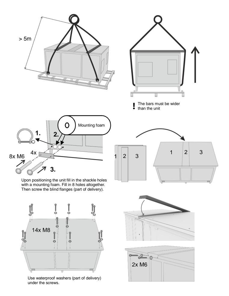
Fit roof cover sheets right after placing the unit in the final installation position. Protect the unit from rough weather (rain, snow) until the unit assembly is complete.
