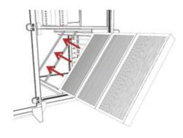
Fitting filters in semicompact unit, front view
