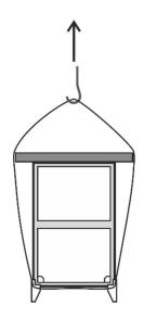
Lift the blocks of semicompact units one after another. Tie up individual blocks from underneath before lifting them.
