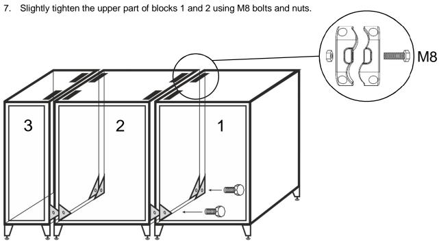
Tightening the unit blocks together
