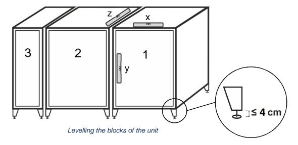
6. Slightly tighten the lower part of blocks 1 and 2 by using M8 bolts together. Use triangle members in inner corners.
