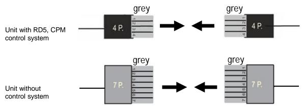
Connect grey connector which powers manometer PMi. Available only for units with RD5 control system.
