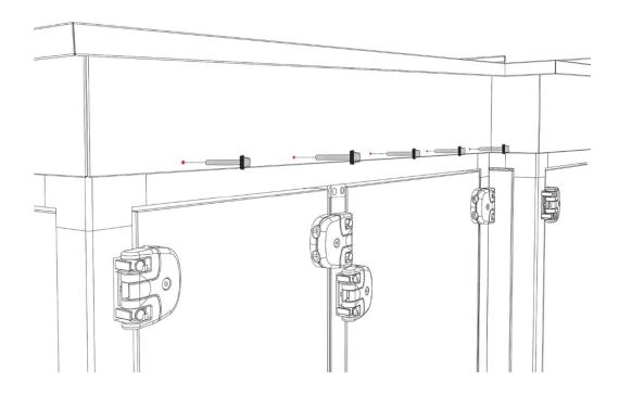
6. Paste silicone into metal U-shaped profiles. Put the profiles onto the connections of roof plates.
