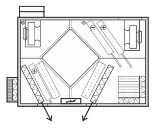
Fitting filters in compact unit, top view
